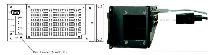
3. While the BLR button is pressed, connect the **power cord** to the keypanel. *KP 32 CLD - Boot Loader Waiting for Download... appears in the display window.*
